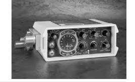
**Principle of Operation:** Time cycled, pressure generator **Power Source for Ventilation:** Dry, oil free, filtered gas:
